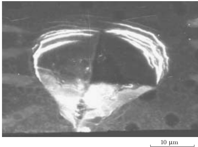
Fig. 1. Deformation pattern in the vicinity of an indentation on the surface of the starting amorphous alloys under an indenter load of 1.5 N.
